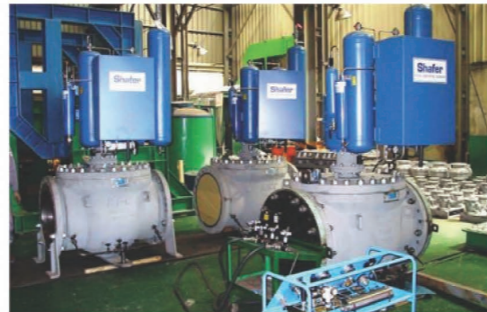
KOC PROJECT 24"-300# RTFE SEATED TOP ENTRY BALL VALVE
